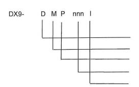
D - pressure measurement devices; L - level sonde
