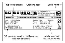
Fig. 1: Example of manufacturing label
