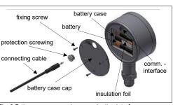
Fig. 3 Battery case cap and communication interface
